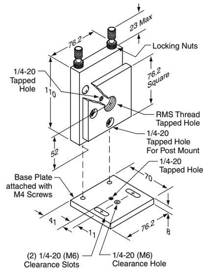
A high resolution unique adjustment system with vertically-mounted controls makes these kinematic mirror mounts particularly valuable for use where access is restricted or where it is necessary to keep the operator's hands away from the optical path, as with high power laser systems. The fine pitch adjusting screws are fitted with knurled locking rings to prevent accidental movement once set in place.
